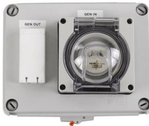
2. For Automatic start attach the 10 metre long generator control cable to the small round two pin plug on the top of the control panel of the generator. It is this cable which will control the starting and stopping of your generator when in the "Automatic" position. The other end of this lead will need to be attached to the small green coloured terminal block in the bottom centre of the IPS unit in the terminals marked NO (normally open) and C (common).
